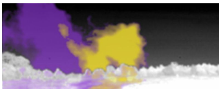
Remote chemical imaging of a simultaneous release of \text{SF}_6 and \text{NH}_3 at 1.5km using the FIRST imaging spectrometer [22]
