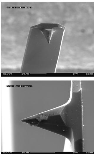
Electron micrograph of a used AFM cantilever image width ~100 micrometers (top) and ~30 micrometers (bottom)
