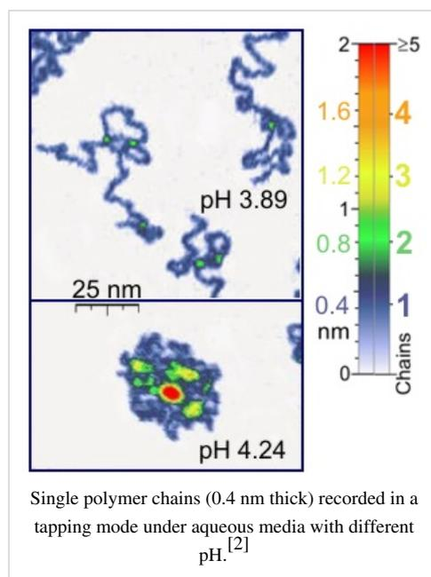
Single polymer chains (0.4 nm thick) recorded in a tapping mode under aqueous media with different pH.<sup>[2]</sup>
