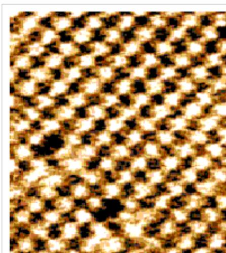
The atoms of a sodium chloride crystal viewed with an atomic force microscope
