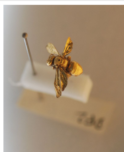
An insect coated in gold for viewing with a scanning electron microscope.
